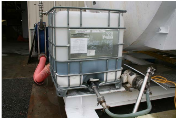
1,000 L HDPE reinforced containers used for storing Phosphoric acid at the local fish oil plant in Cordova. These containers could be used in order to improve digester support.
