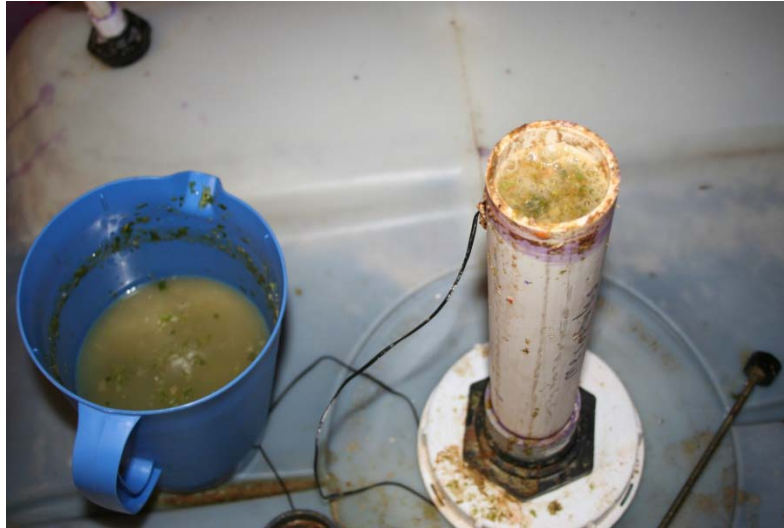
Figure 7. Common overflows following a typical feeding regiment of 1kg food + 1kg water. The PVC inlet tube does not allow for easy use of a funnel and it is hard (especially for students) to observe an overflow prior to it occurring. Issues with sanitation result as many of the digesters exhibit this problem. Clogging continues to slow the feeding process and will need to be improved in the project future.
