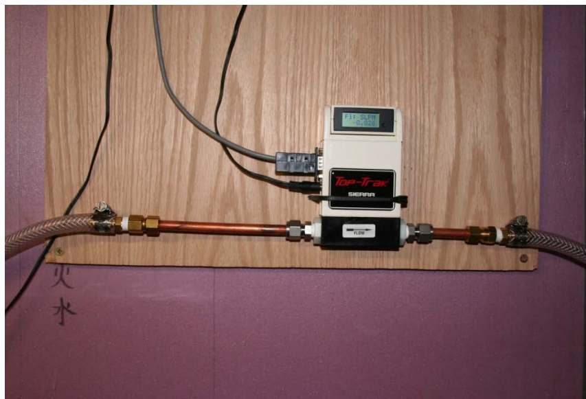
The old connections pictured above used cloth reinforced rubber tubing to connect the gas flow meters though the transducer (bottom) is intended for pipe fittings to be installed. The length installed upstream of the device is intended to allow for uniform flow that is not turbulent, causing a misread by the device.
