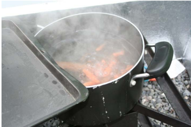
One gallon of boiling water is used to illustrate biogas usage as a cooking fuel. The modified stove pictured sustained a constant flame with a burn rate of about 300 L/hr.
