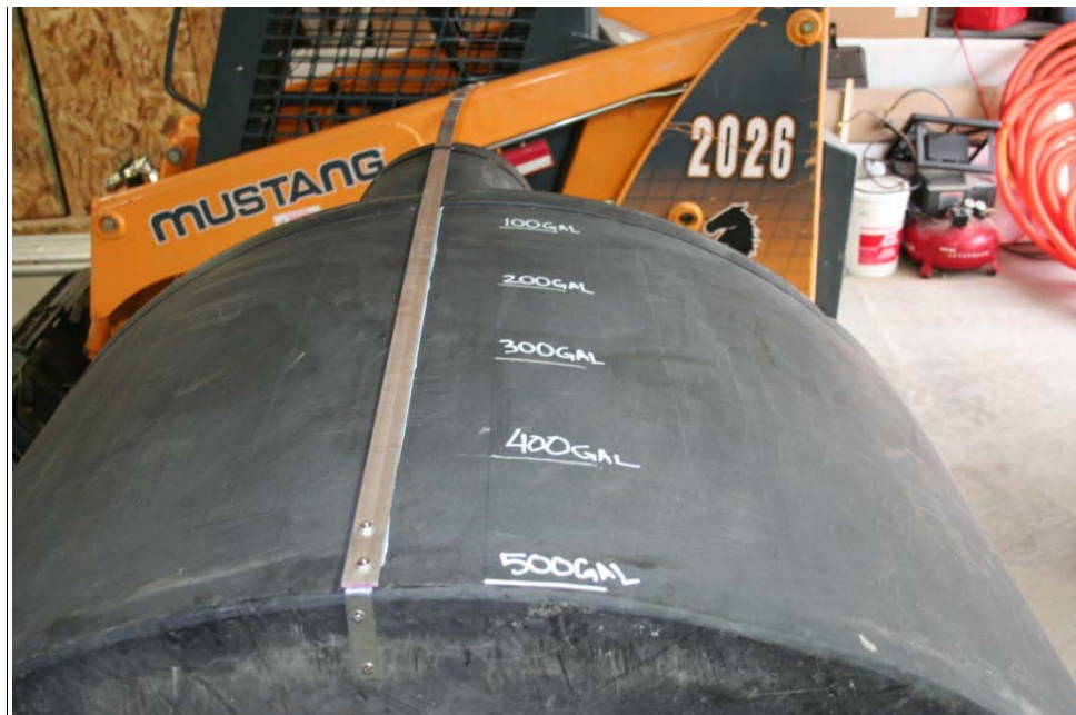
The gas storage vessel was calibrated and given indication markings for how much gas is stored inside. The aluminum bar attached to the tank is used as a level indication that can be viewed once the tank is fully assembled. This looks great, Casey!
