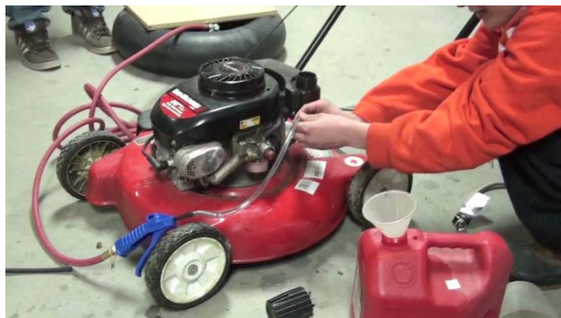
Students rig a common lawnmower to run off of biogas.
