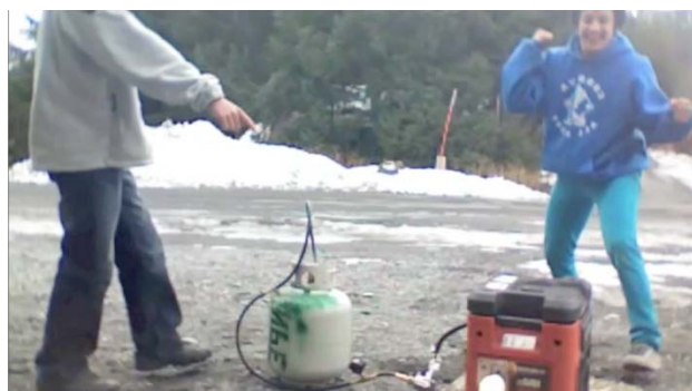
A 4-cycle 1850 Watt Husky generator was converted to run on biogas and other available gaseous fuel types. Here students celebrate as the generator successfully starts using propane.
