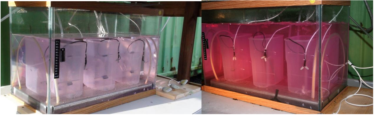
Figure 5. Installation and deployment of the wet-cup flux traps at the Cordova digester site earlier in the project. Automated bubble traps were installed on 10/15/2010 in an effort to monitor total gas flux from digesters 1, 4, 5, and 6 in a to the Sierra Top-Trak 820 Mass Flow meters
