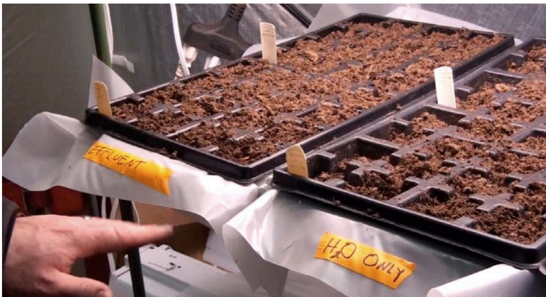
Lilly starts contained within the greenhouse aim to see if effluent samples grow faster or slower given the same conditions as starts with only light and water inputs with minimal nutrient content
