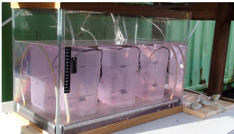
Automated bubble traps were installed on 10/15/2010 in an effort to monitor total gas flux from digesters 1, 4, 5, and 6 in a to the Sierra Top-Trak Mass Flow meters
