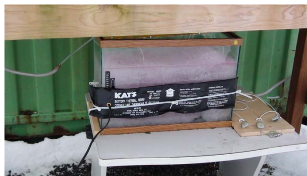
Aquarium pictured here with a car battery jacket in an effort to thaw out the tank. The jacket worked very well and is now used periodically to prevent freeze up.
