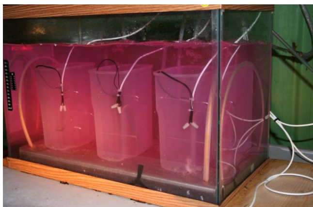
Here the water traps are observed in action during one of the four daily pressure releases of tanks 1, 4, and 5. Tank 6 (on the right) has not demonstrated gas production since the water trap was installed.
