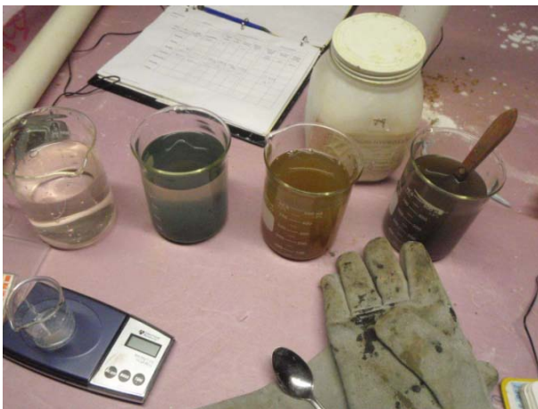
Testing acidic effluent for amount of mediating chemicals needed to be added.
