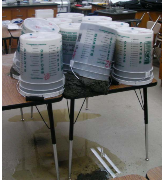
Figure 1. Buckets #1-8 and 10 in the 25°C room, showing exploded buckets #1 (back left) and #2 (front) on November 28, 2009.
