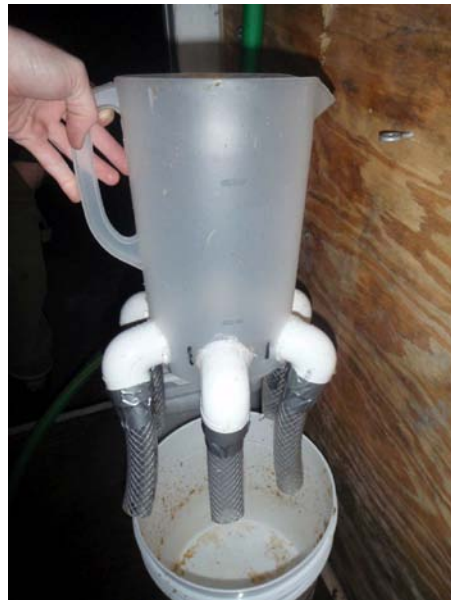
CDHS student-designed food dispersal system, to insure even distribution of food batches.
