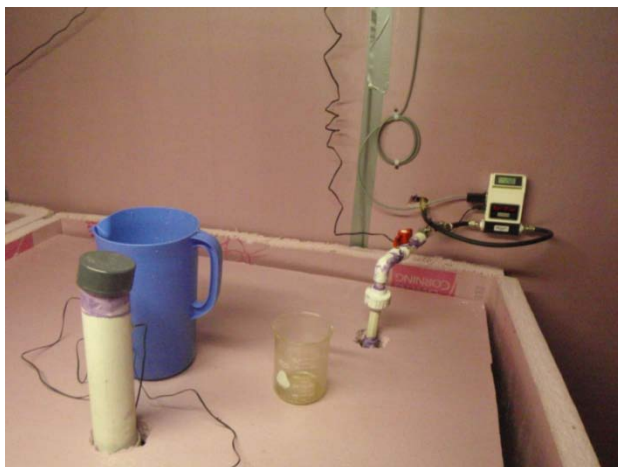
Complete digester set-up, with feeding pitcher, effluent test beaker, and running flow meter.
