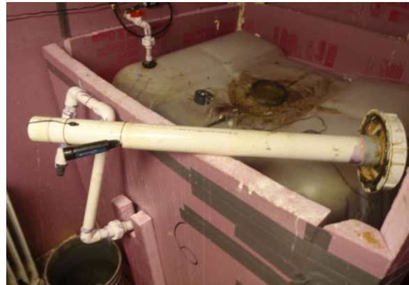
Feeding tubes are fit with internal temperature dataloggers.
